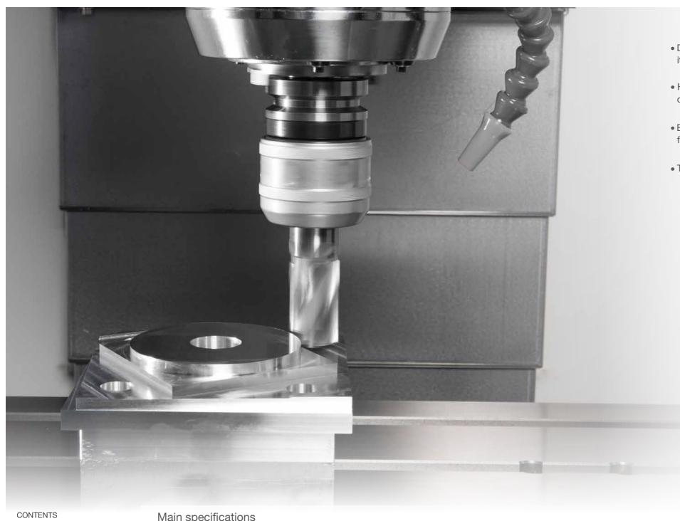
• Direct-drive spindle with dual-contact system provides excellent machining quality and efficiency.
