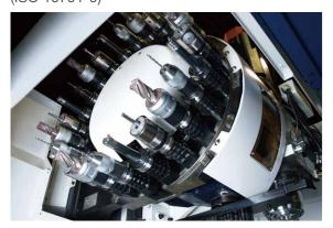
Adopts encoder in the cam box for ensuring the signal transmission is quick and stabile. With Tongtai PLC logic setting, ATC will re-try which reduces the possibilities of machine stop when errors happened during tool changing.
