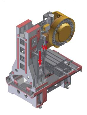
High efficiency flushing system allows the chip removed rapidly, especially suitable for aluminum machining.
