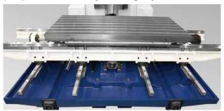
The Y axis employs four guideways to offer superior support of the X axis saddle and best accuracy.
