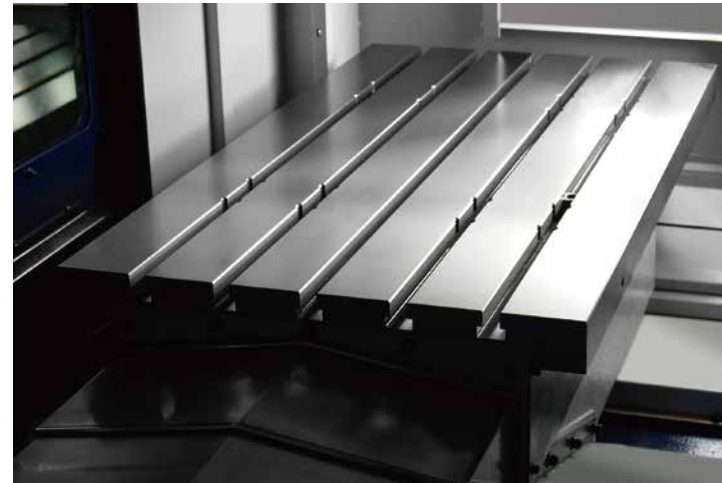
Fine ground table surface with excellent flatness.
