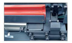
POWERFUL REMNANT EXTRACTION SYSTEM WITH SELF-CEN-TRING CLAMPING JAWS
