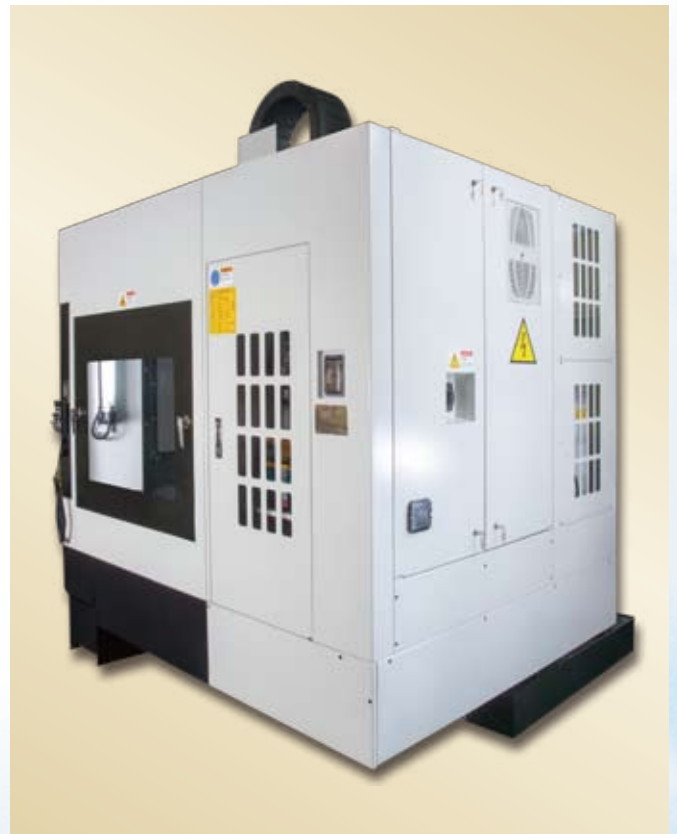
▲ Full guarding covers oil cooler, transformer, pneumatics etc. on rear side for clean environment and easy maintenance.
