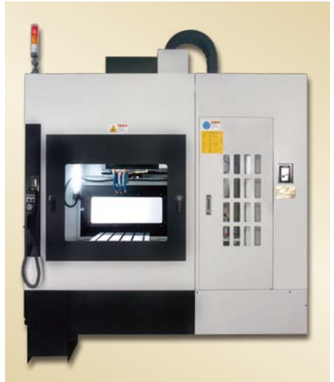
▲ Right side big window for big long work piece in & out.
